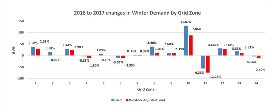
Note that the large percentage increase in Grid Zone 12 is primarily due to more positive load values in Kumara (KUM0661), which was largely negative due to elevated levels of embedded generation in 2016.
